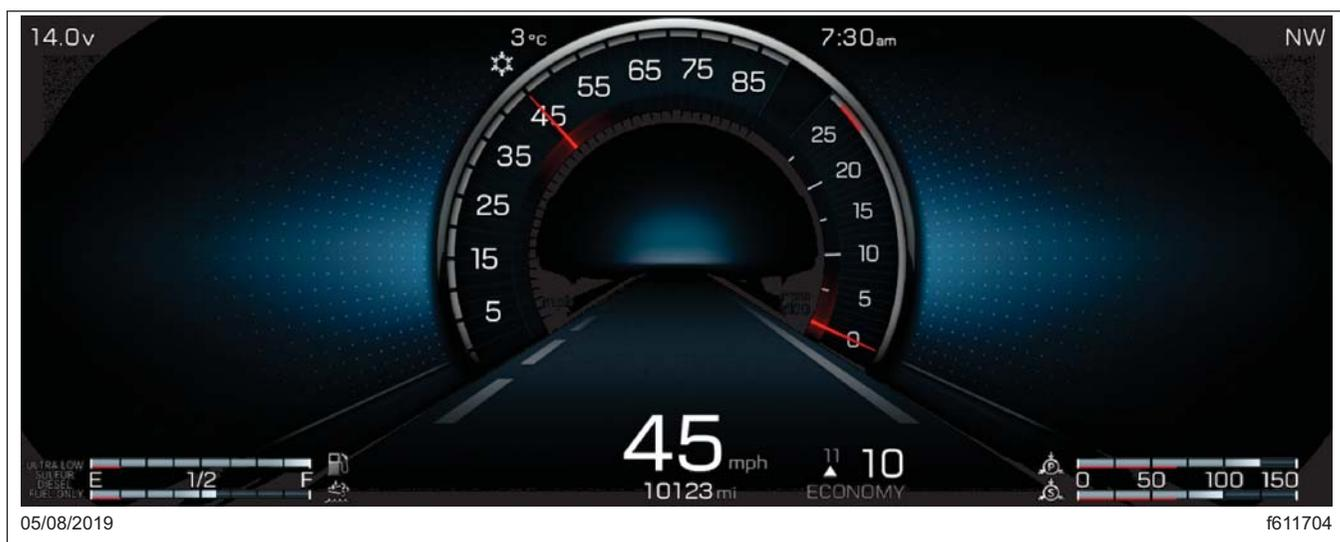
**Fig. 3.49, Driver Display Base Screen - ICC5**
