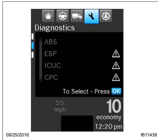
**Fig. 11.2, Electronic Control Unit (ECU) List in the ICUC**
