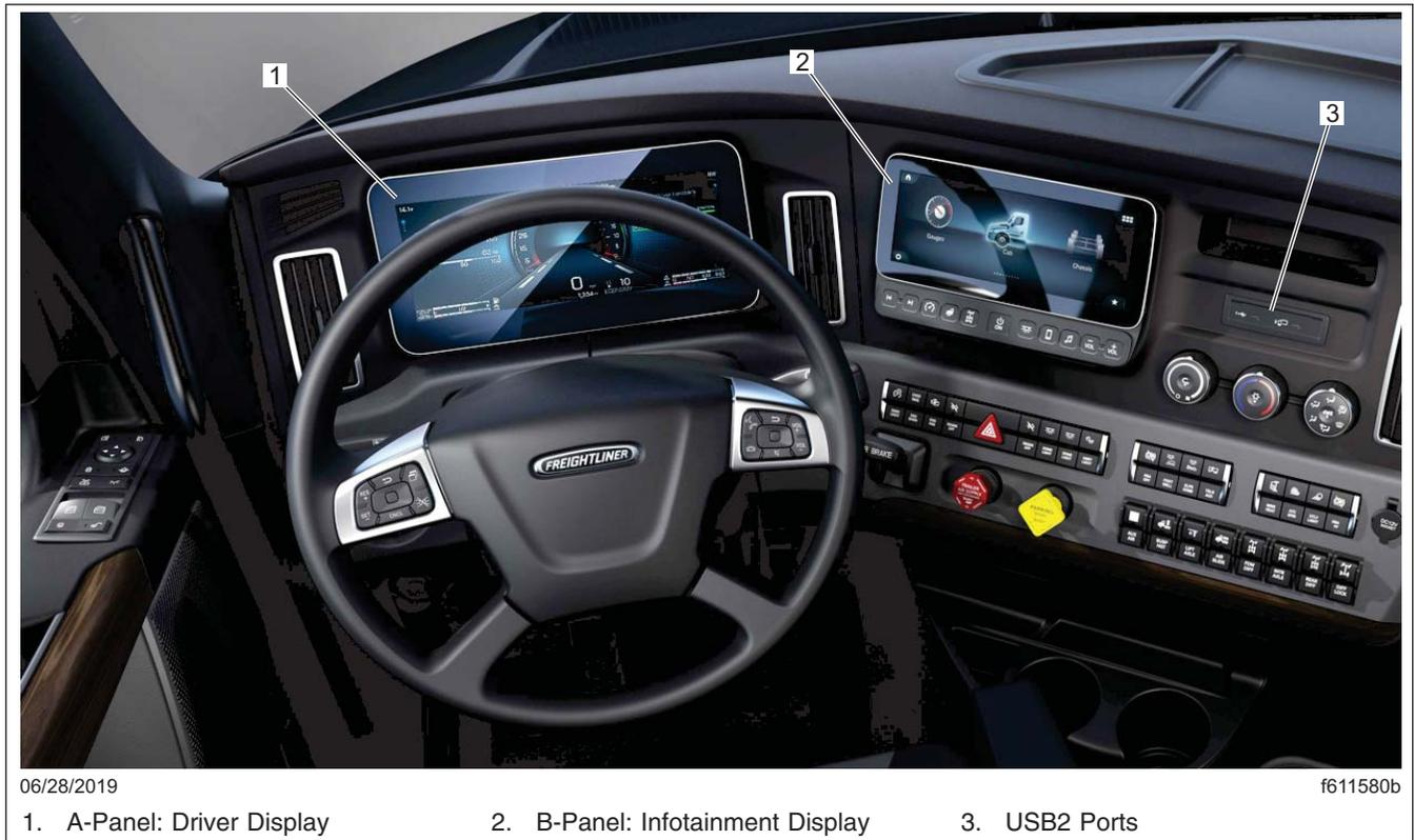
**Fig. 3.48, ICC5 Dual Display Screens and USB2 ports**
