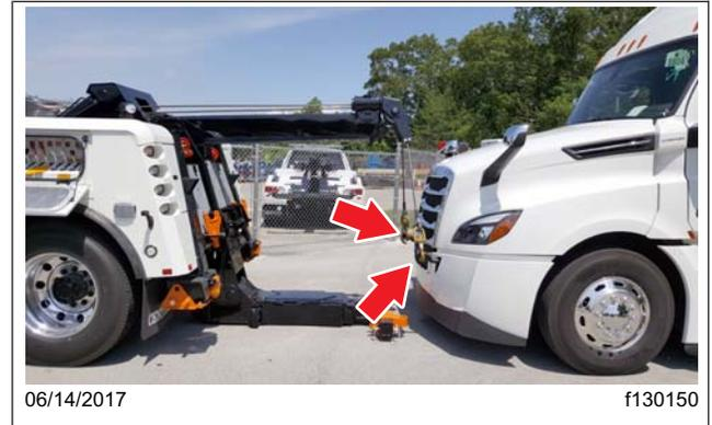
Fig. 26.7, Tow Cables Connected to the Tow Hooks
