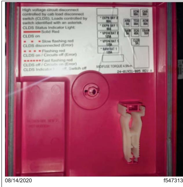
**Fig. 11.6, Example Fuse Labeling on BCA Cover**
