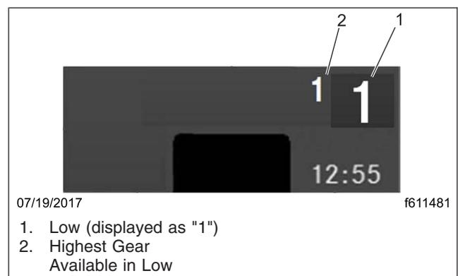
**Fig. 17.13, Allison Gear Display in Low Gear**
