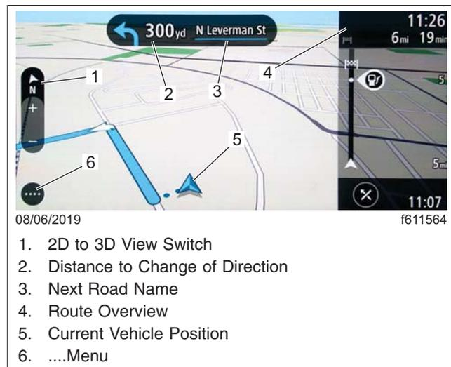
Fig. 7.12, Overview of 3D Display- ICC5
