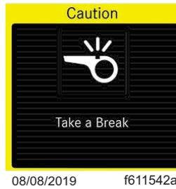
**Fig. 6.26, Attention Assist Warning Lamp - ICUC**
