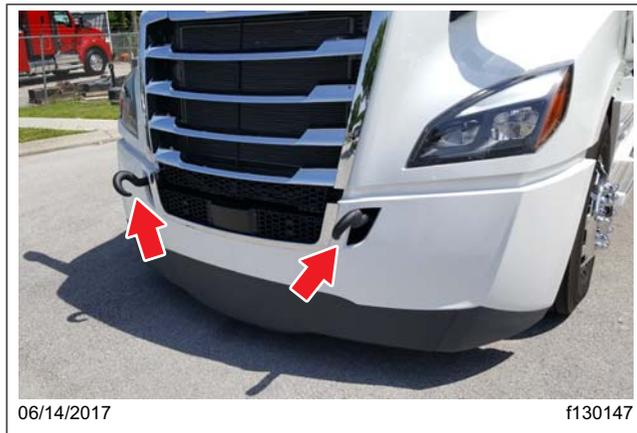
Fig. 26.5, Tow Hooks Installed, Facing Down
