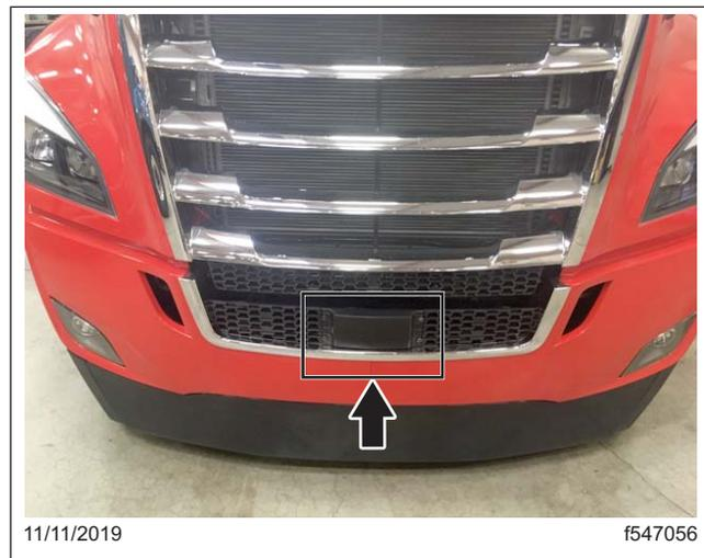
**Fig. 6.2, Forward Radar Location**
