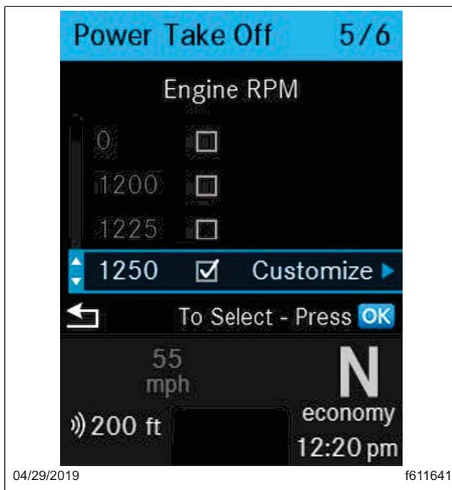
**Fig. 3.22, Quick Access Screen: Power Take Off (PTO)**
