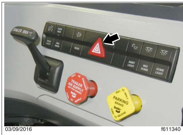
**Fig. 4.4, Hazard Warning Switch**
