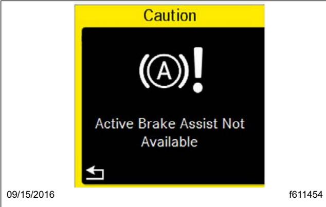
Fig. 6.7, Active Brake Assist (ABA) Alert - ICUC
