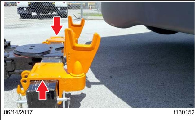
Fig. 26.9, Lift Adaptors Installed on the Crossbar
