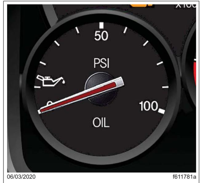
Fig. 3.39, Analog Engine Oil Pressure Gauge - ICUC
