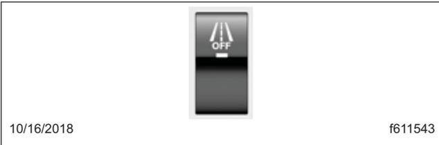
**Fig. 6.23, Active Lane Assist Switch**
