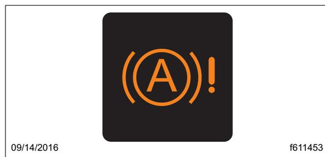
**Fig. 6.6, Active Brake Assist (ABA) Indicator Lamp**
