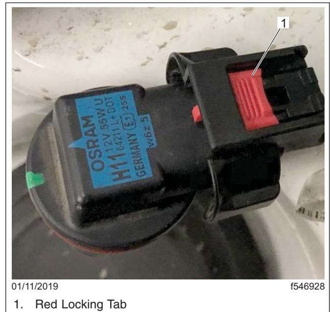
**Fig. 22.6, Halogen Headlamp Electrical Connector**
