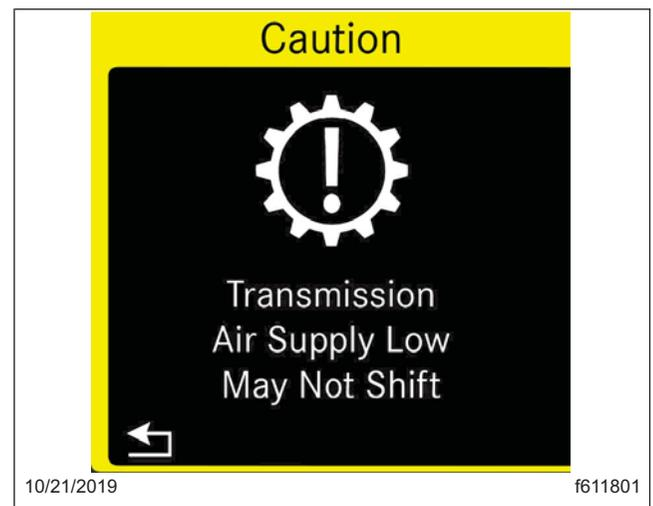
**Fig. 17.8, Low Transmission Air Pressure Pop-up**
