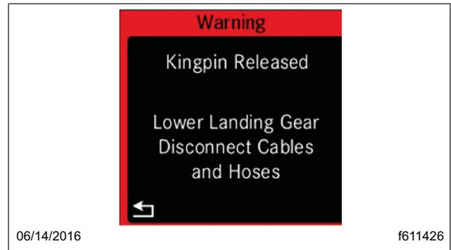
Fig. 20.10, Kingpin Release Alert Screen
