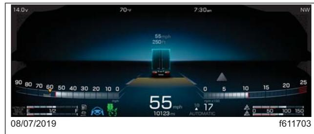
**Fig. 3.50, Driver Display Pilot Screen - ICC5**
