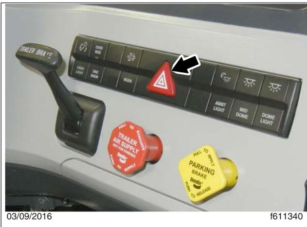
Fig. 26.1, Hazard Warning Switch
