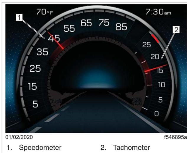
**Fig. 3.59, Speedometer and Tachometer Base Driver Display Screen - ICC5**
