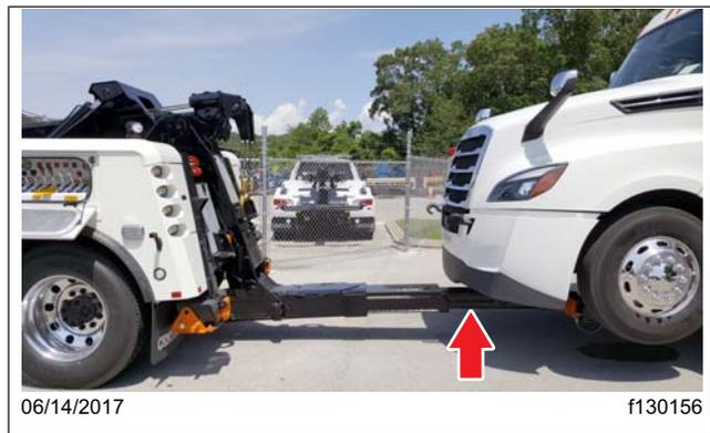
Fig. 26.13, Retracting the Recovery Boom
