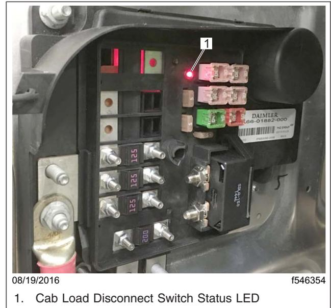
1. Cab Load Disconnect Switch Status LED
